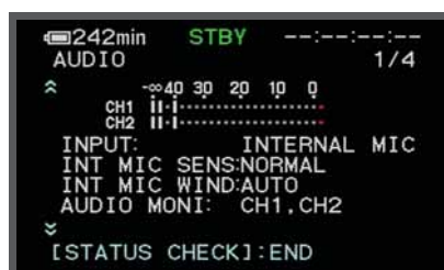
2-channel Independent Audio Record Level Control with Audio Level Meter
